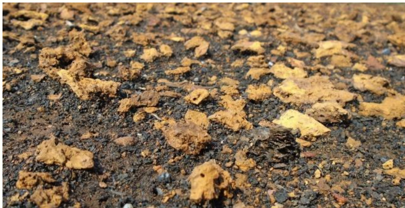
Figure 4. Bog iron ore found close to soil surface (image taken from: https://www.haraldthesmith.com/wp-content/uploads/2018/02/OreHeader.jpg )
