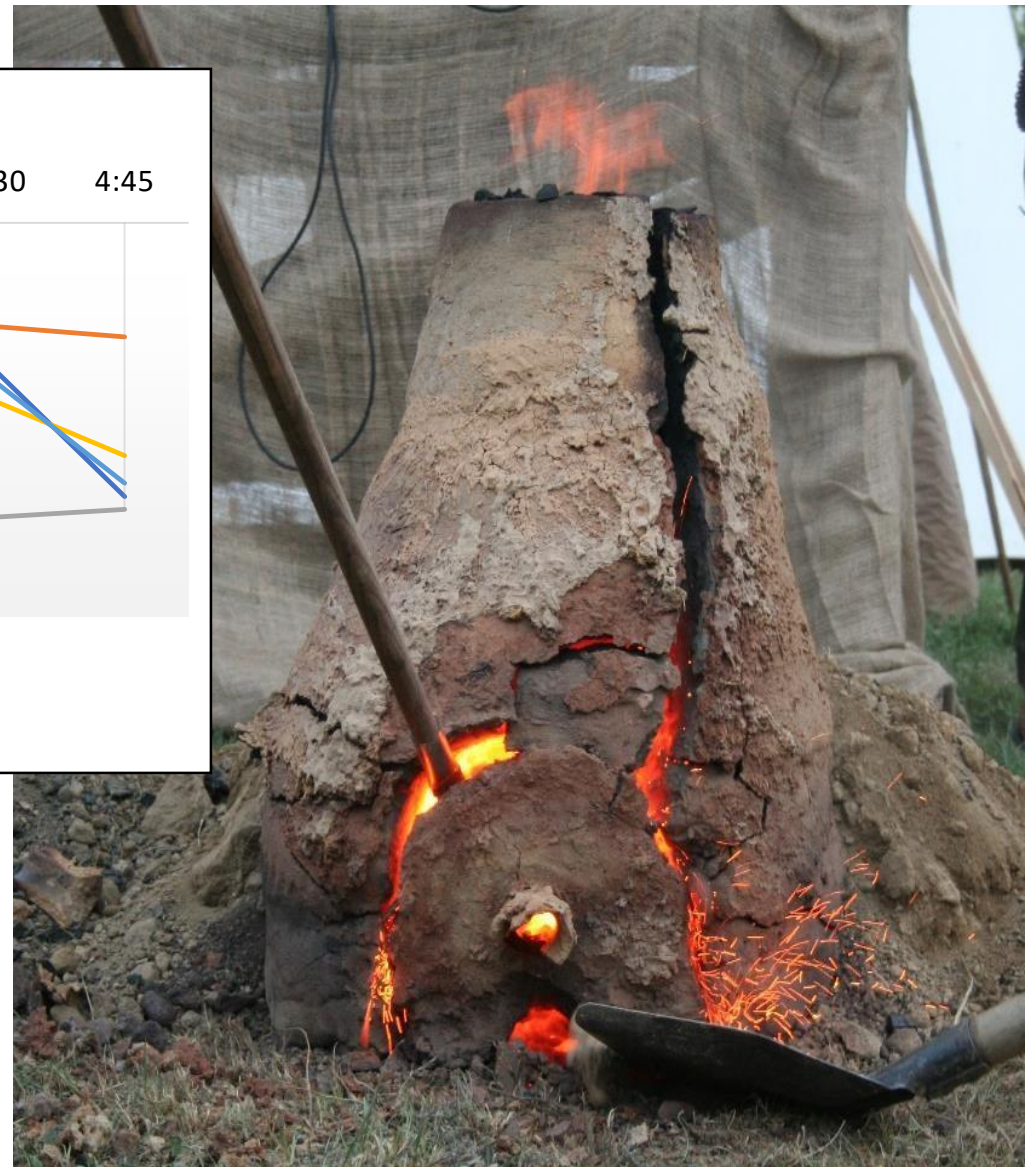
Experimental iron ore smelting in a free standing furnace, Koprivnica 2019.
